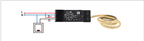
Push调光【连接示意图】 Push Dimmer Connection diagram
