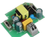
筒射灯内置认证驱动（拨码调色温调电流） The built-in certified driver of the downlight (dip to adjust CCT and current)
